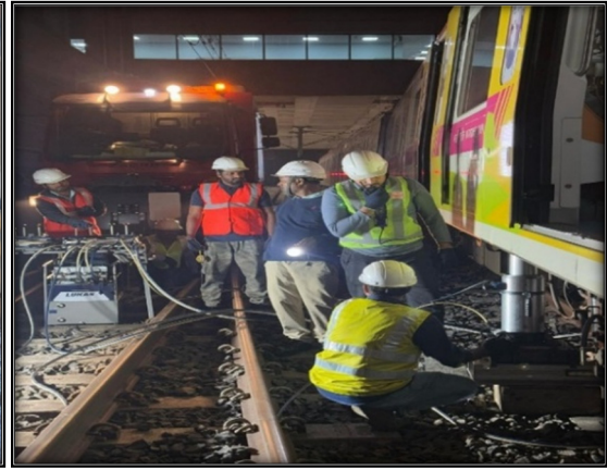
Lifting of train for Re-railing.
