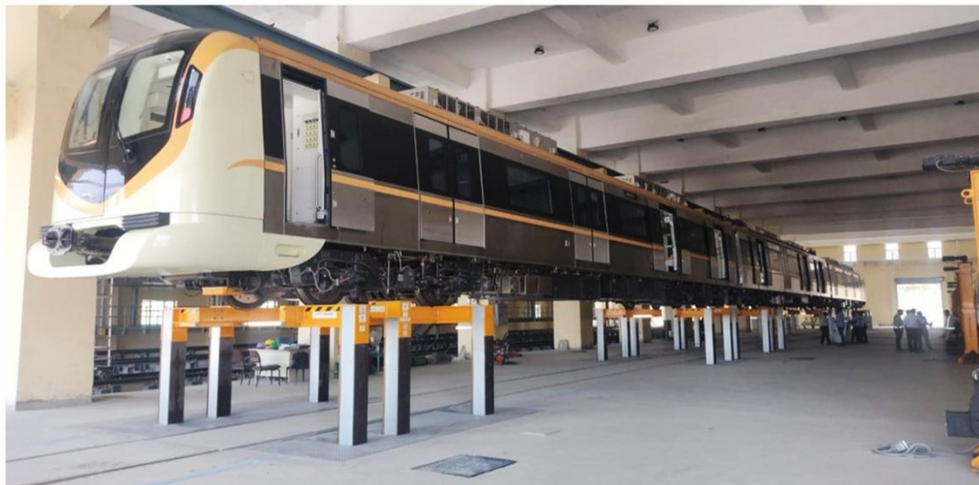
Train Maintenance on Under Floor Lifting System at Hingna Depot
